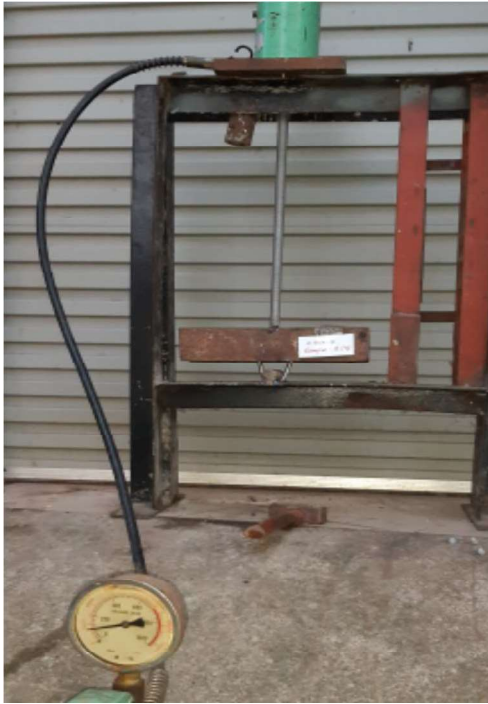
Sample 2a – Reading 1400psi
